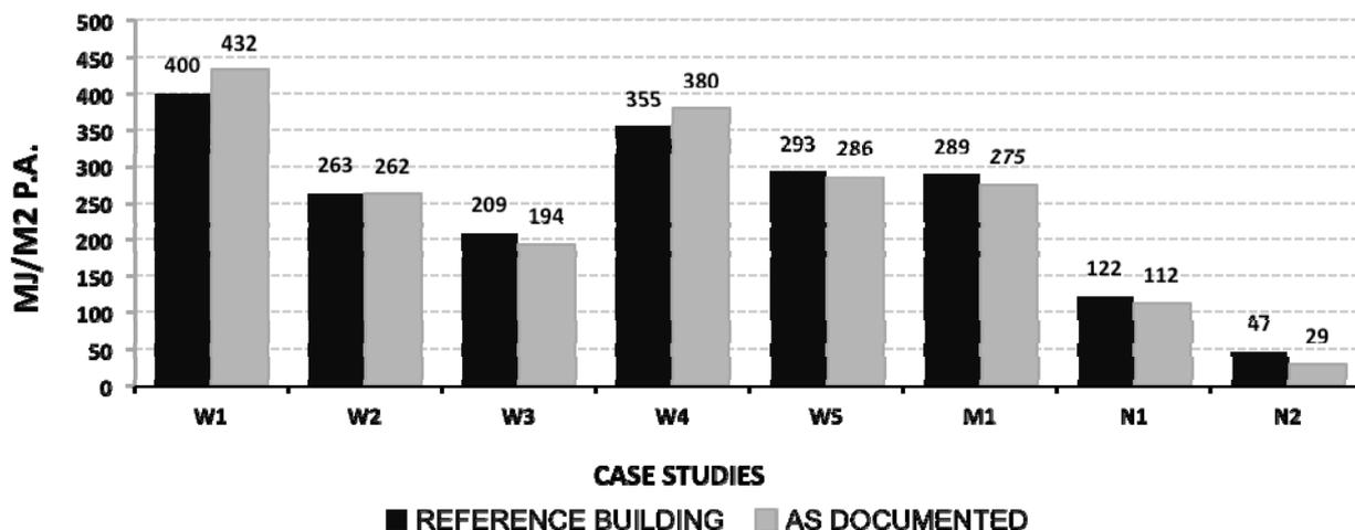
Figure 2: Comparison of the total annual energy required for space heating and cooling for the NZS 4218 reference design and as-documented design of case study houses
